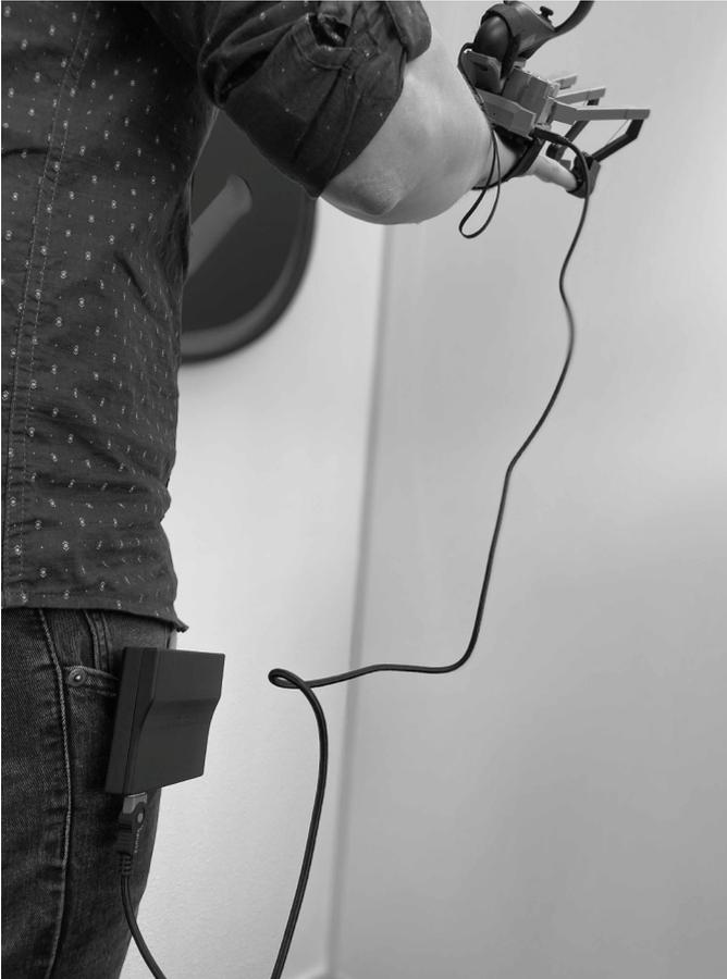
The back of the wireless kit has a clip. Preferably, the wireless kit should be strapped to the front or back pocket of your trousers.
